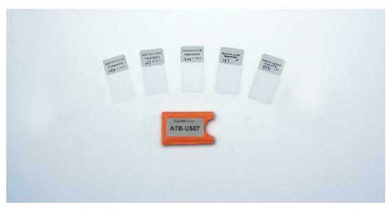
• covers the range from 20 up to 2000 µm, with < 3 % tolerance
